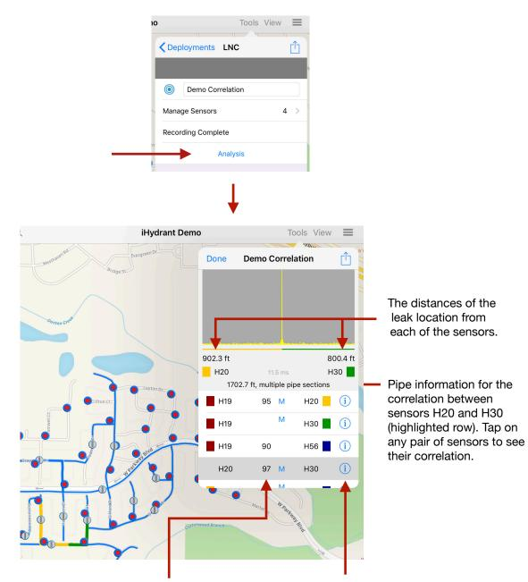
The number between the two sensors is the Correlation Score (in this case, "97", from a range of 0 - 100). The higher the score, the stronger the confidence of a leak at that location.
