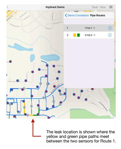
Tap on the 2nd Pipe Route to see the alternate pipe paths and possible leak location.
